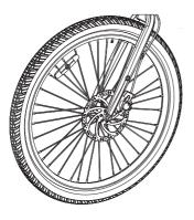
**Caution:** Never touch the brake rotor, especially when the wheel and/or bike is in motion, or serious injury could occur. Hand oils can cause squeaking and decrease brake performance.
