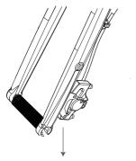
B. Remove the plastic insert card from the front brake caliper.
